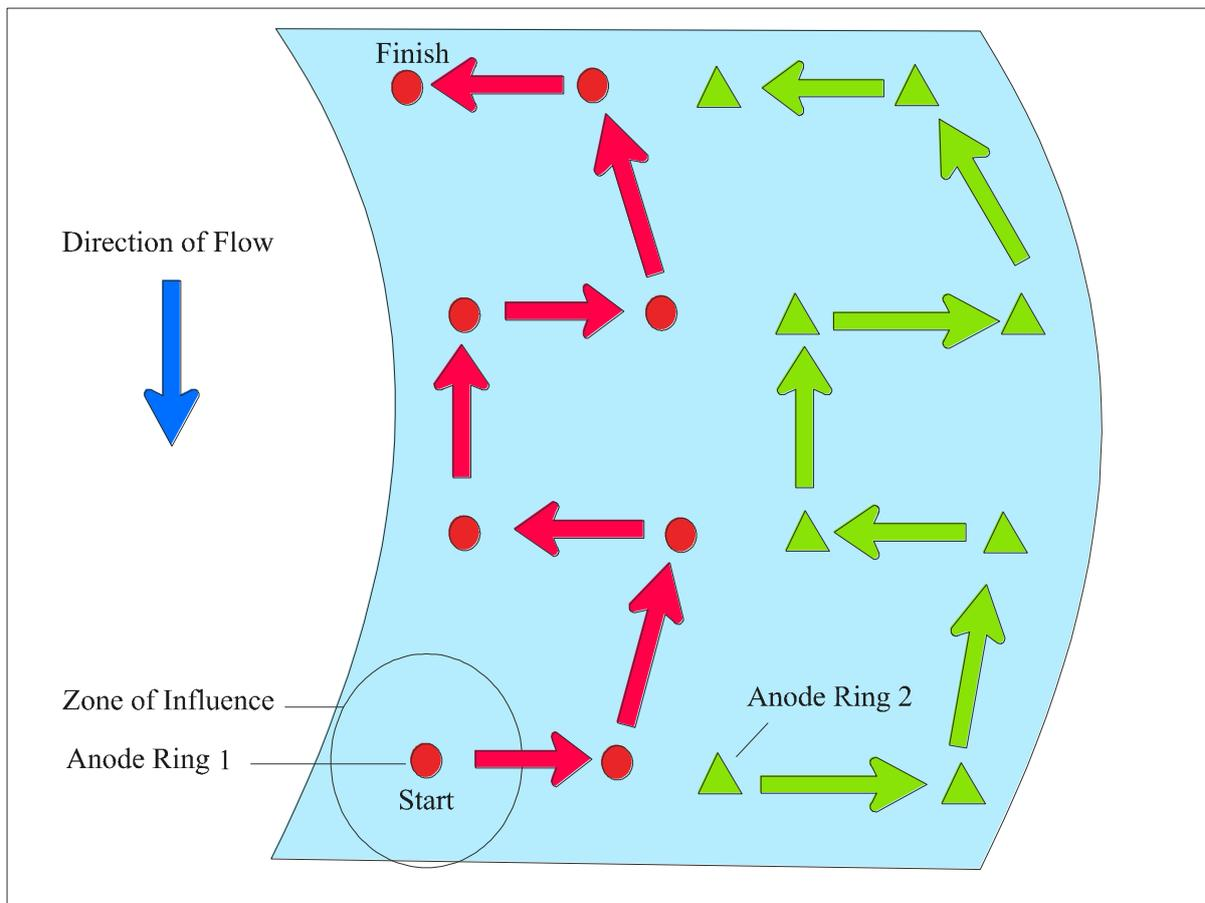
Figure 6. Movement of two anodes working as a team in a larger river
