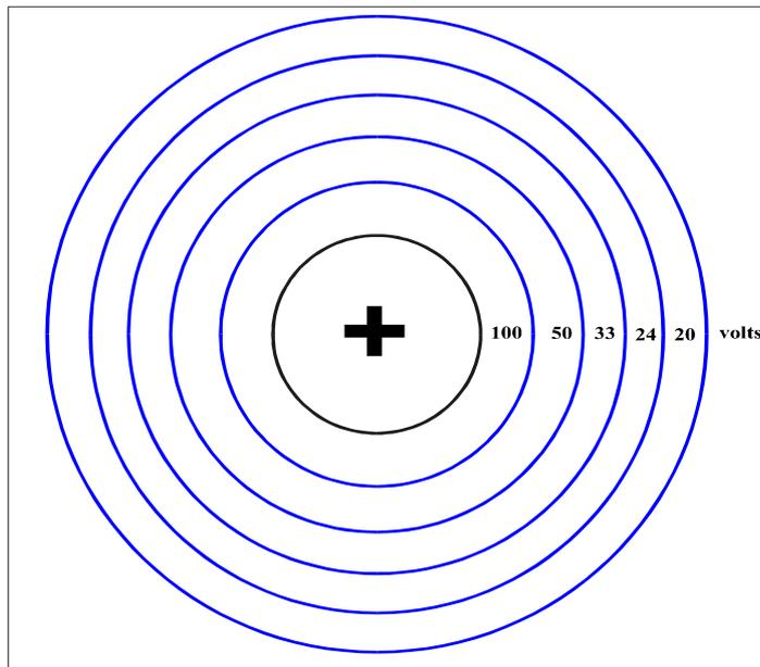
Figure 3. Constant voltage lines around an anode ring
