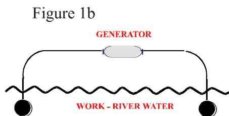
For both safety and to enable choice of electricity types, the power source for electrofishing comprises both a portable generator (either batteries or engine) and a control box. Two electrodes are needed as a minimum to complete the circuit. In DC fishing the positive electrode is hand-held and it is known as the anode. The negative electrode, the cathode, is physically different and is often a metal plate or braided copper strip. These typical components are shown in Figure 2.
