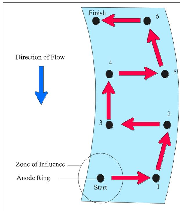
Figure 5. Movement of a single anode across and up a small river
