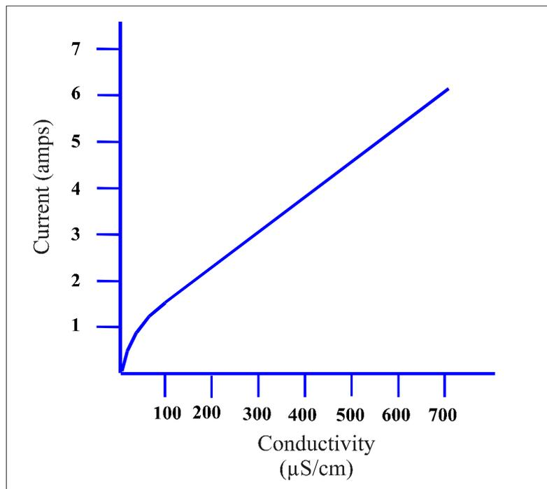
Figure 7. Current passed between two electrodes with increasing conductivity
