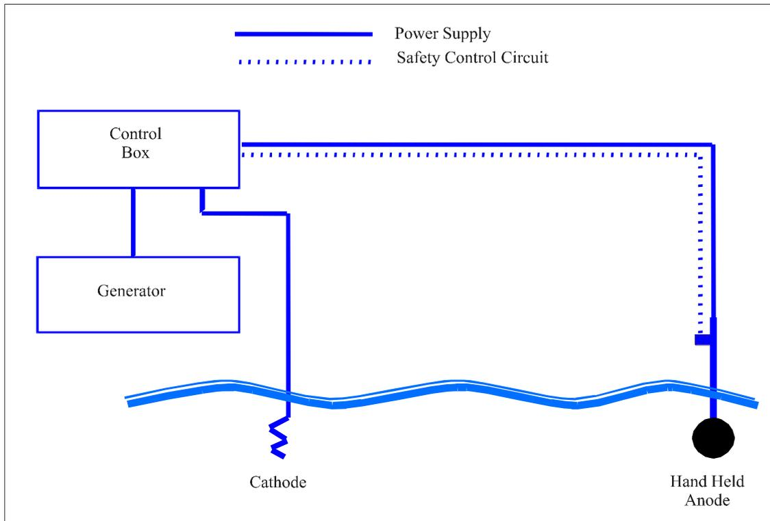
Figure 2. Typical components of electrofishing equipment
